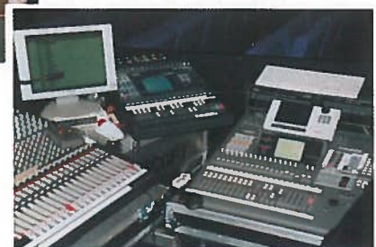
Right, the Yamaha O2R and O3D mixers controlling the sound effects and band mix
